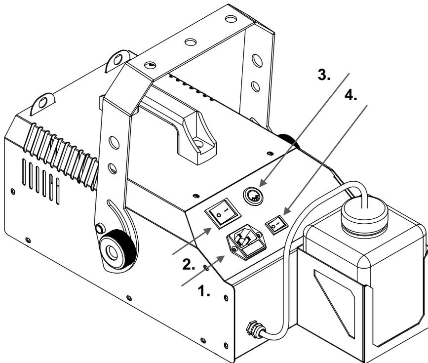
**1. POWER:** IEC mains power input socket with fuse holder for F6,3A 250V fuse.
