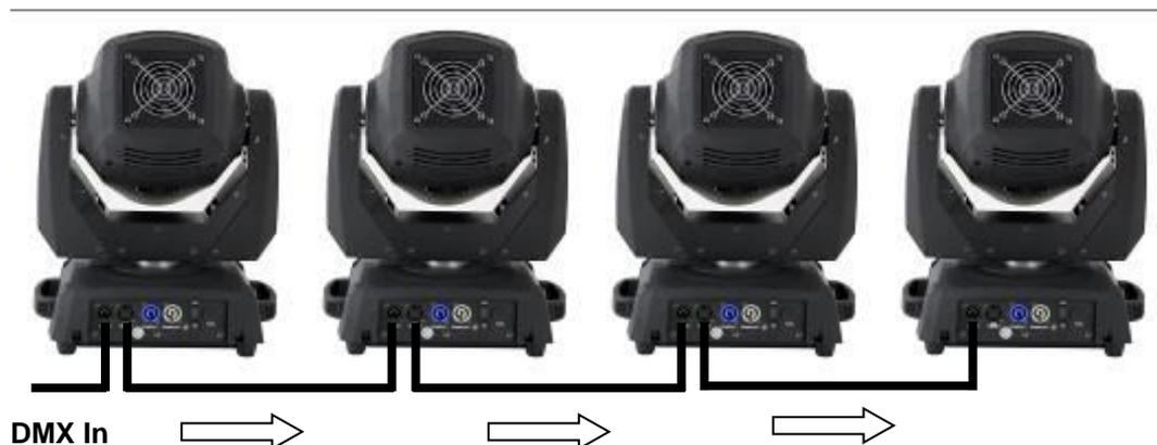
For systems with very long DMX cable runs or high electrical interference, such as in a discotheque, it is recommended to use a DMX terminator. The DMX terminating resistor is implemented in an XLR connector as a 120  $\Omega$  resistor between pin 2 and 3, which is plugged into the last output socket of the DMX line.
