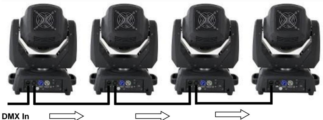
For systems with very long DMX cable runs or high electrical interference, such as in a discotheque, it is recommended to use a DMX terminator. The DMX terminating resistor is implemented in an XLR connector as a 120  $\Omega$  resistor between pin 2 and 3, which is plugged into the last output socket of the DMX line.
